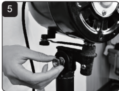
5 Desparafuse o motor
