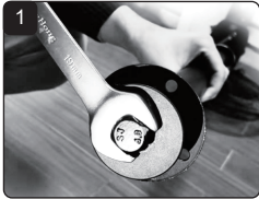
1 Remove the screws from the screw motor
